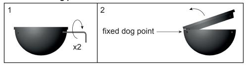
3. Screw the arms into the half-sphere. The curved part of the arms has to be parallel to the ceiling and in the alignement of the half-sphere. Screw the set screws into the half-sphere to avoid unscrewing.
