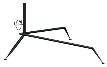
3. Unpack the end of the arms to fit them to the central mast. Remove the cable protective caps in red plastic from the tubes. Release the packaging of reflectors without removing it completely.
