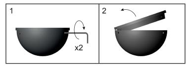
3. Screw the arms to the half-sphere. Screw the set screws in the half-sphere to avoid unscrewing.
